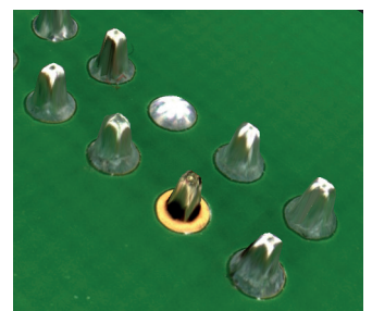
Insufficient wetting (front) and missing pin (back)
