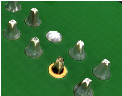
Insufficient wetting (front) and missing pin (back)
