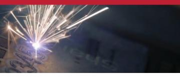
Unique properties characterize these fiber lasers, such as electrical-optical efficiencies up to more than 30%, outstanding beam quality with M2<1.1 for single-mode fiber laser design, M2<1.2 for double-clad fiber, a long lifetime (> 100,000 hours) and a compact, maintenance-free and insensitive design.
